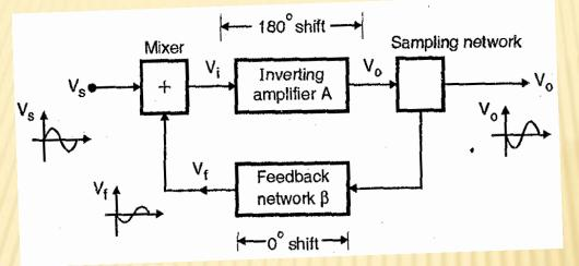
The block diagram of an amplifier with a Negative Feedback Fig.
